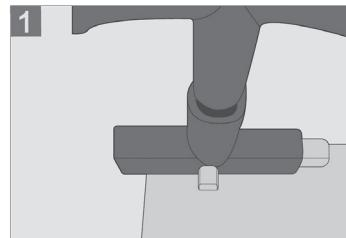
2. The adjustment from the handle is made according to the width of the tile to be broken.
