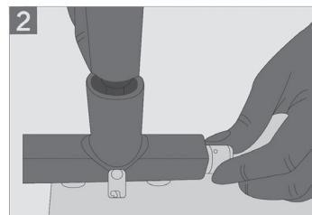
3. Work can be done more efficiently and quickly by simultaneously applying force with the T-handle and the upper and lower handles.
